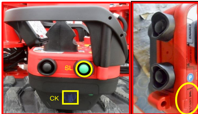
Picture 8a: start/link button on radio control.
