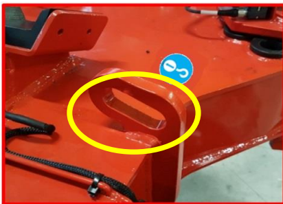
Picture 16: hooks for sling and transport.
