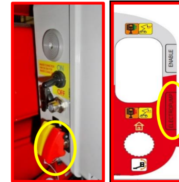
Picture 29: electropump activation buttons.
