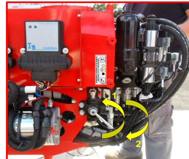
Picture 30: electropump tap.
