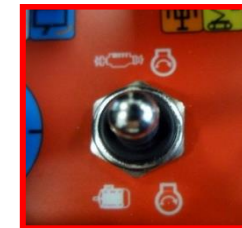
Picture 5: power on/off lever on the radio/wired control.
